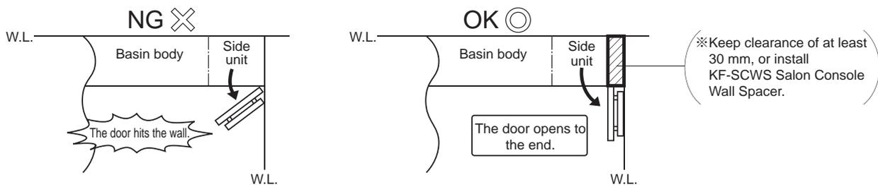
※The illustration above shows when installed at the right corner. (Same as when installed at the left corner.)
